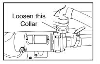
and air to escape from the pumps and related plumbing. Then, retighten the collars.
